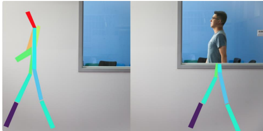
Human Pose estimation using radio signals in 2~5GHz [1]
